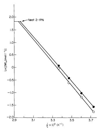
Figure 1 Natural logarithm of the equilibrium monomer concentration ln[M]<sub>e</sub>, as a function of the inverse of the ceiling temperature,  $1/T_c$ : ( $\bigcirc$ ) toluene; ( $\bullet$ ) tetrahydrofuran
